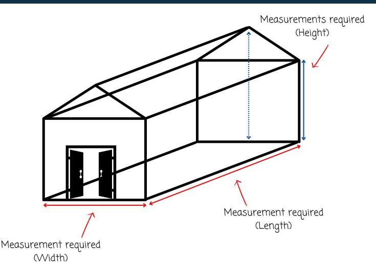
If you have a pitched roof, it is important to provide us with two height measurements. One from the floor to the eaves (solid blue line) and one from the floor to the apex of the roof (dotted blue line).
