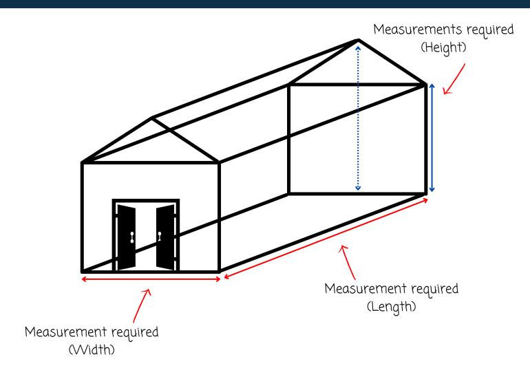
If you have a pitched roof, it is important to provide us with two height measurements. One from the floor to the eaves (solid blue line) and one from the floor to the apex of the roof (dotted blue line).
