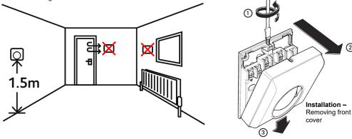
Mounting and wiring the thermostat to a standard single recessed metal box.
