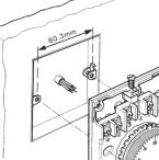
Mounting and wiring the thermostat to a standard single recessed metal box.
