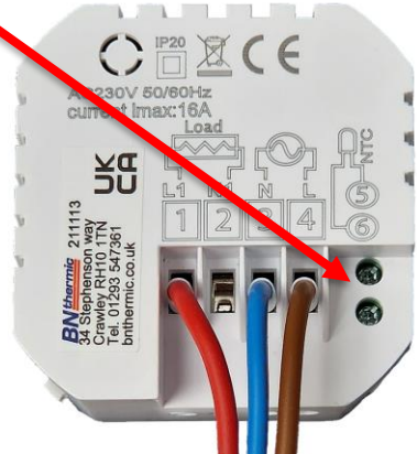
Back view of thermostat mounted on the lid
