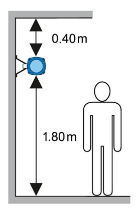
Please Note – The 1.80m mounting height is the minimum recommended height if you wish to mount high on a wall, are not using the protective guard and people are present.
