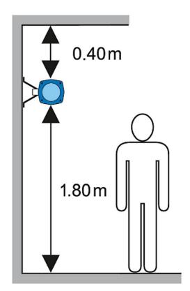
Please Note – The 1.80m mounting height is the minimum recommended height if you wish to mount high on a wall, are not using the protective guard and people are present.
