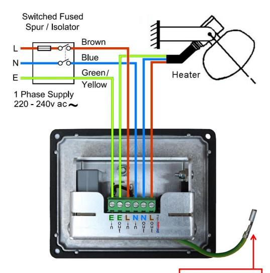
Before refitting the lid this Earth lead MUST be reconnected to the back of the box.
