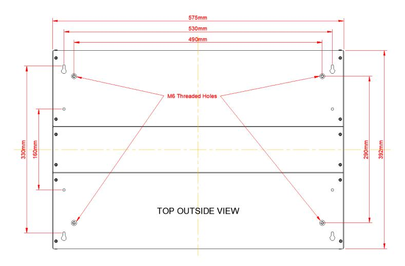
Using the drawing to the left mark out the holes required to secure the heater case to the ceiling. Use the 4 x keyhole slots and an additional 2 holes once installed to lock the heater in place. These addition 2 holes must be used to stop the possibility of the case sliding off its fixings.
